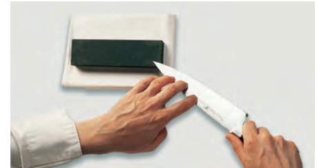
(a) Hold the knife firmly. Start with the tip of the knife against the stone as shown, and hold the edge against the stone at a 20-degree angle. Use the guiding hand to keep an even pressure on the blade.
