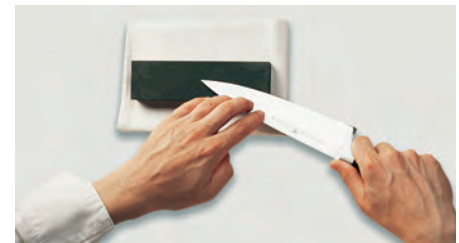
(b) Start to draw the knife over the stone. Press very gently on the blade.
