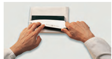
(d) Draw the knife across the stone all the way to the heel of the blade.
