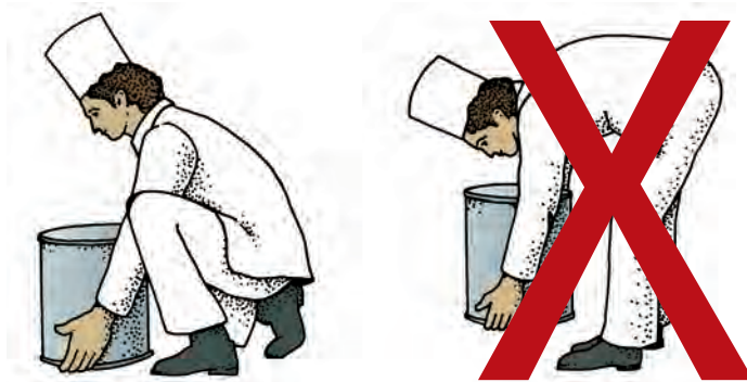
(a) Squat on one knee, and then lift with the leg muscles. (b) Do not bend over and lift with the back.
