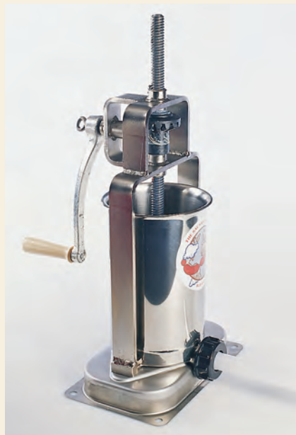
(a) A small sausage stuffer fitted with a medium nozzle. This stuffer holds 5 lb (2.3 kg) of meat at a time.
