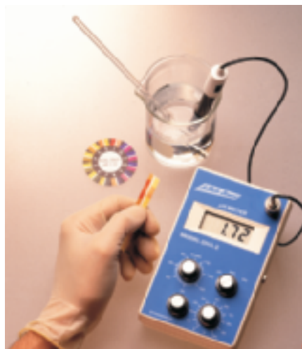
Figure B.13 Both pH paper and a pH meter can be used to determine the pH of a solution. The meter will give the more precise reading.
